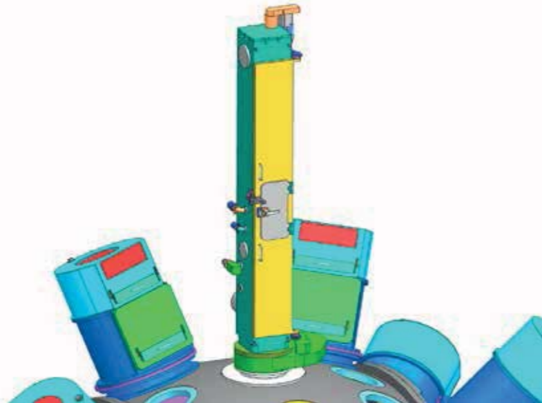
Model showing position of the Target Inserter in the Orion Target System and statistics.
